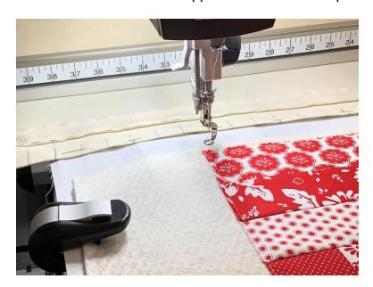
When you look at the computer screen the crosshairs of the needle are not at the top of the grid. They are way down into the design. The Safe Area needs to be realigned.
