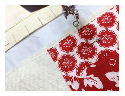
Set the Safe Area when Q-matic is opened or use the Set Safe Area icon on the lower left. Make sure both the X and the Y belts are engaged. The Safe Area should be 1-3 inches larger than the quilt top on all sides. Move the sewhead all the way back and to the left of the quilt top. Note: the quilt top is not right at the top of the Safe Area at this time. Press Set on the sewhead.
