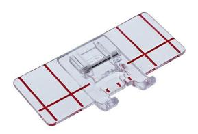
horizontal red line matches the needle drop so you can line up the start of each row. The small red mark denotes the center of the design for lining up with the marking for the first row. ( Perfect for this week's project.)
