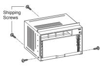
Slide the unit from the cabinet by gripping the base pan handle and pulling forward while bracing the cabinet.
