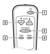
Energy Saver - In this mode the compressor and fan turn off when the set temperature is achieved. Approximately every 3 minutes the fan turns on to allow the unit sensor to accurately determine if more cooling is needed.
