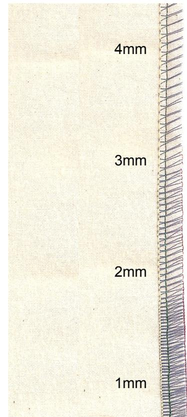
Stitch length adjustments may be needed to accommodate thicker or thinner threads or different weights of fabric. General guidelines for stitch length settings:
