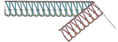
Examine your 4-thread sample. The illustrations below show examples of unbalanced stitches and how to correct the settings to balance the stitch. When making corrections in the tension settings, increase or decrease the settings as needed, moving the dial ½ to 1 number at a time. Stitch a seam using the new settings and then evaluate the new stitch. Continue in this manner until the stitch is balanced.
