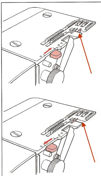
The Rolled Hem Selection Lever moves the stitch finger in and out of position.
