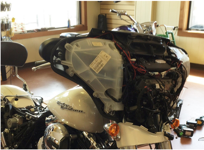
Remove outer fairing., and speaker enclosures.
