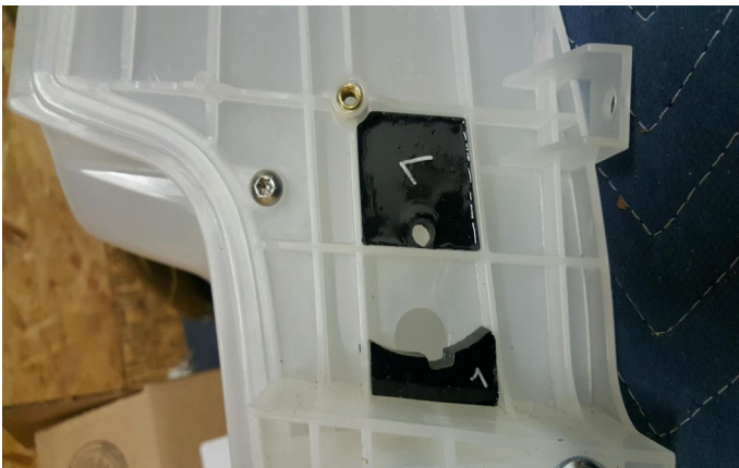
Test fit templates. Prepare to drill pilot holes.
