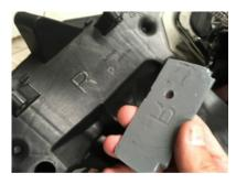
Using the drill templates, drill pilot holes in the enclosures.
