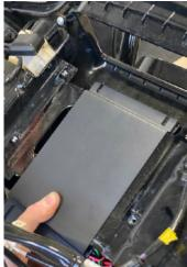
Locate the four holes in the bottom of the amp. Secure the amp with the provided short black screws and washers. Blue Loctite® is advised. Screw are in the Moto720 Box, washers come with the RG15 Bracket.
