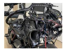
Remove the old speakers from the enclosures saving the screws and set aside speaker leads with the Molex connectors.
