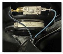
Secure the new Speaker, Spacer and Spacer Ring Assembly with the supplied screws. Drive the NEW supplied screws into new locations in the pods. Do not reuse the existing holes.
