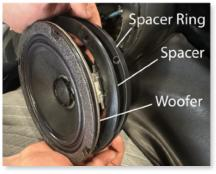
Connect the speaker leads to the new woofers as shown screws. DO NOT CROSS THE POSITIVES AND NEGATIVES. If your woofers are out of phase, you will have no bass.
