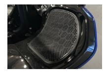
Remove the speaker enclosures, radio and any other audio equipment.
