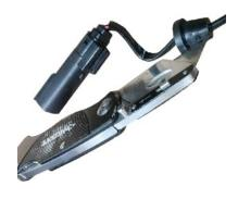
Route the SinisterSound woofer leads through the original grommet hole and into the speaker enclosure. Reuse the grommet and seal with glue.
