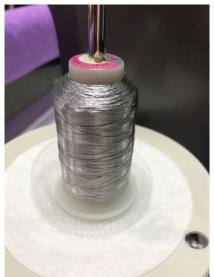
This is a thread net folded in half and mostly tucked up inside the cone to make a bowl where there are no exposed edges of the netting that might catch the thread.
