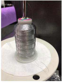
Threads like this metallic want to unwind and "puddle" around the bottom of the spool. With the Innova, the disc below the thread prevents it from catching on the bottom of the cone.
