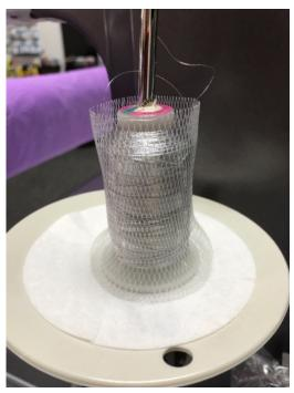
This is the WRONG way to use a thread net, it will add drag and tension to the thread as it comes off the spool.
