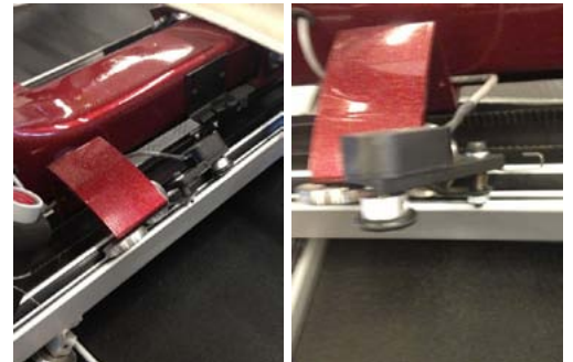
Encoder in proper position on left, encoder released from spring on right.
