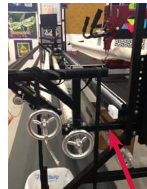
The entire pivotal access assembly is attached to the table leg at this point. These side brackets hold the pivotal access assembly and backing bar.
