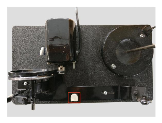
This handy little thread clipper can be used on the front of your bobbin winder, or attached to the backside of the head of your long-arm sewing machine.
