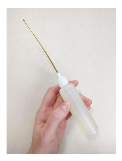
This needle-tip oil bottle is extra handy for oiling your bobbin hook assembly.
