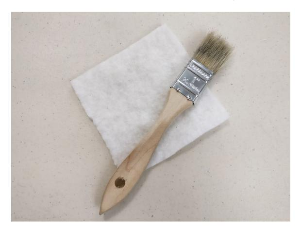
A small brush like the one shown above can be used along with a scrap of batting to brush off lint from the sewing machine head, especially in the bobbin hook assembly. This can be a critical part of keeping your machine running smoothly!
