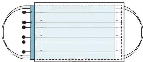
Following the direction of the arrows on the template, bring the end of each arrow to its arrowhead, creating three pleats. Pin the pleats in place along the mask sides.
