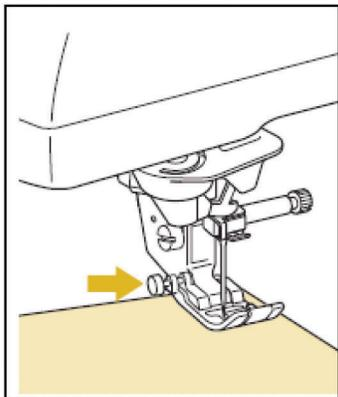
3. Release the black button. The presser foot remains level, enabling the fabric to be fed.
