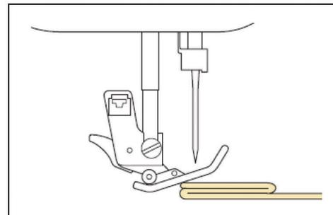
If the presser foot is in the up position, and you are sewing heavyweight or multiple layers of fabric which do not fit easily under the presser foot, use the presser foot lever to raise the presser foot to its highest position. The fabric will now fit under the presser foot.
