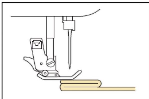
**Note:** Once the trouble spot has been passed, the foot will return to its normal position. When "Automatic Fabric Sensor System" (Automatic Presser Foot Pressure) in the machine settings screen is set to "ON", the thickness of the fabric is automatically detected by the internal sensor so the fabric can be fed smoothly for best sewing results.
