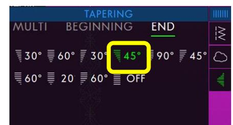
19. Engage **Needle Down**. Stitch this program until it stops keeping the outer edge of the **8-Maxi Foot** along the edge of the card. The machine will automatically do the tapering and stop at the end of the program.
