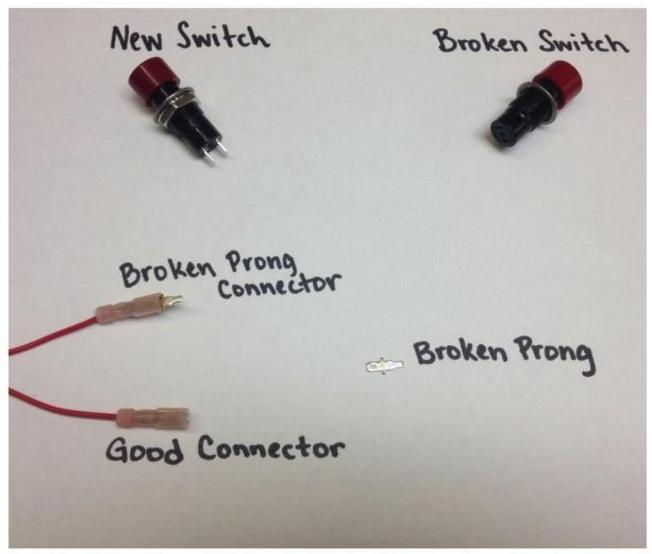
As seen in the diagram the prongs often get pulled out with the connectors when changing switches. In order to fix this carefully pull the prong out of the connectors with pliers. When changing switches in the future carefully wiggle the switch instead of pulling when removing the connectors.
