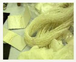
The filaments are carded or reeled to form yarn, which starts out coarse and stiff due to the residual sericin—a gummy substance excreted by the silk worm during its spinning process.
