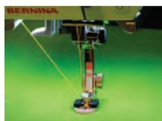
The newest version of Button Sew-On Foot #18 has a non-slip sole to make it even easier to sew on buttons by machine. This short little foot sits on the button and has an adjustable shank that creates room for the button to go through the buttonhole, even on thick fabrics!
