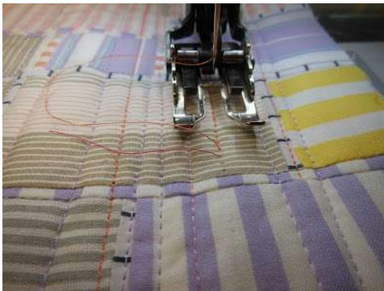
Put a new bobbin in. Now grab the loop of top thread and stick your finger into the loop so the takeup mechanism won't pull it taut.
