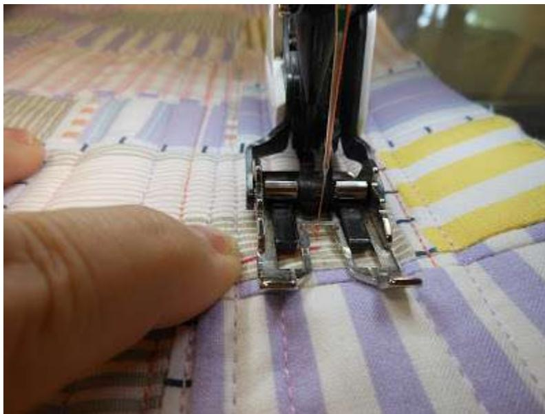
Lower the presser foot so the needle is exactly in place to continue the stitch line. Holding the thread ends taut with your finger, start stitching again.
