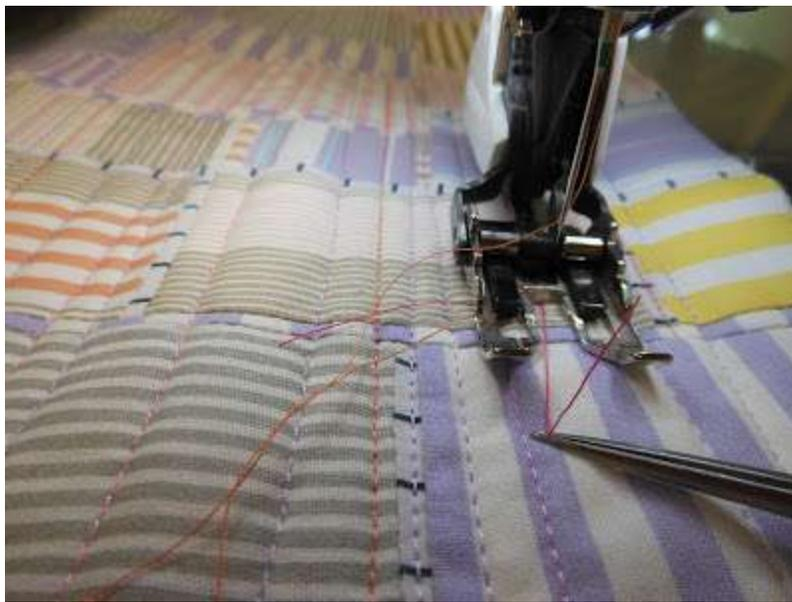
Pull the thread end over to the side, along with the thread end from the old bobbin and hold them both firmly with your finger so they won't escape. With your other hand, grab the top thread on top of the sewing machine, somewhere between the spool and the tension plates, and pull it backwards so the thread is taut between the quilt and the needle.
