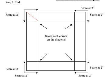
After scoring, fold the diagonal corners inwards and adhere to the inside. Make sure to also place glue on the outside of the corners. See diagram below. Place a paperclip on each corner and set aside to dry.
