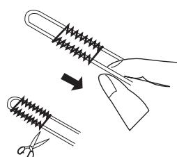
1 With the buttonhole foot raised, hook the filler cord on the spur at the back of the foot.
