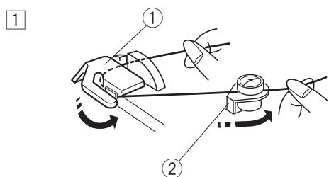
① Hold the thread with both hands and pass the thread under the thread guide.
