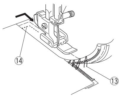
5] Raise and release the foot, and re-attach it with the left side pin.
