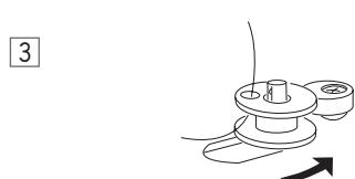
③ Push the bobbin winder spindle to the right.
