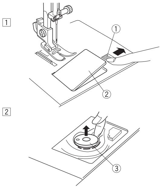
① Push the hook cover plate release button to the right and remove the cover plate.
