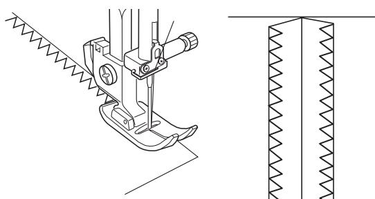
The zigzag stitch is used on the seam allowance to prevent fabric from fraying at raw edges.
