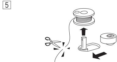
⑤ Start the machine again. When the bobbin is fully wound, it will stop automatically.
