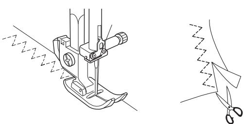
This stitch is used to finish the seam allowance on synthetics and other fabrics that tend to pucker. Place your fabric to allow a 1.6 cm (5/8") seam. Trim the seam allowance after sewing.
