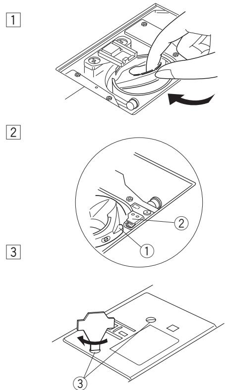
① Insert the bobbin holder into the hook race.
