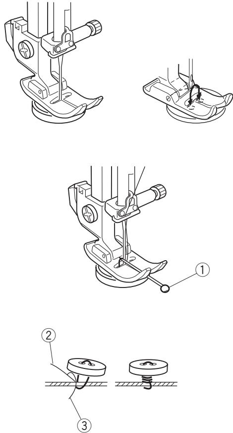
Unthread the needle. Adjust the stitch width to match it with the span of the holes in the button.
