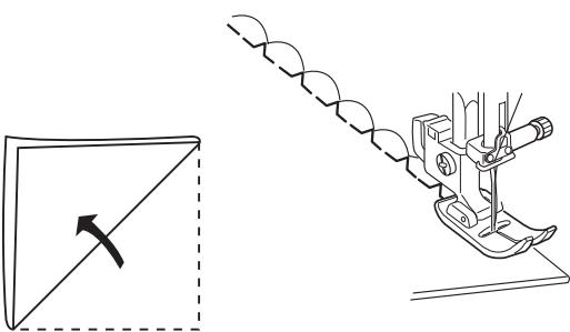
Place the folded edge along the slot of foot. The needle should fall off the edge of the fabric on the right forming a tuck.
