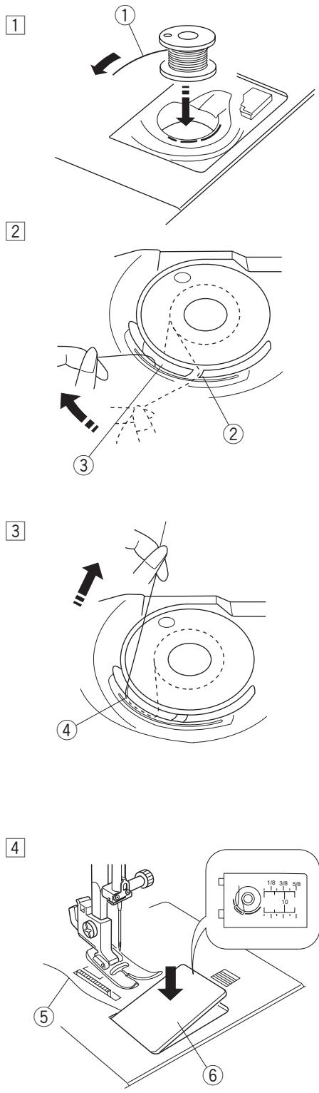
**[1]** Place the bobbin in the bobbin holder with the thread running off as illustrated.
