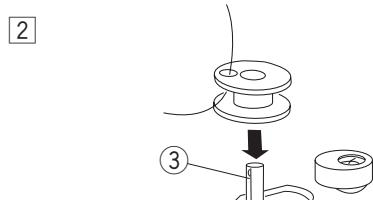
② Pass the thread through the hole in the bobbin from the inside to the outside.
