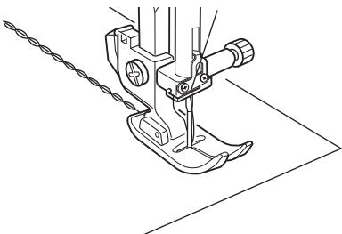
The pattern is sewn with two stitches forward and one stitch backward, forming a seam that does not rip easily. Use it to reinforce areas such as crotch and armhole seams.
