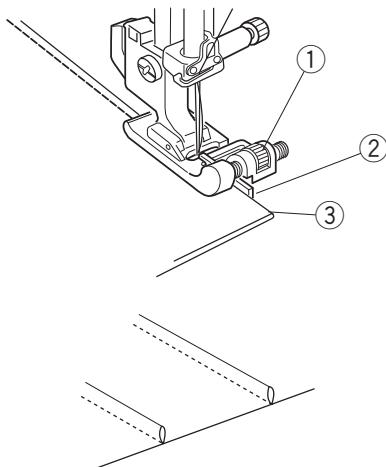
Fold a fabric wrong side together and Lower the needle into the fabric 0.1 – 0.2 cm inside the folded edge. Lower the foot and turn the screw to align the guide on the foot with the folded edge. Sew slowly while guiding the folded edge along the guide.
