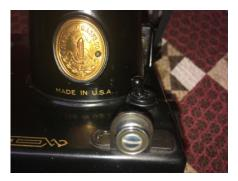
"<u>Speckled</u>" Tension disc. On certain machines of this era you'll find a speckled Tension knob disc vs the standard black used from 1933 through 1957. In this case our "Crinkle" has it.
