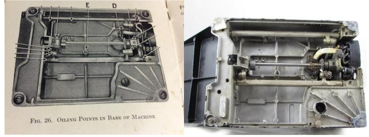
One last detail view of the bed casting area beneath the motor is shown below for comparison. As with the entire main bed casting and folding extension table, standard production Featherweights have circular casting features as highlighted in the right hand photo. The unique machine described in this article does not have them. You may have also noticed casting surface roughness throughout in comparison to the smoother finish on normal production Featherweights.
