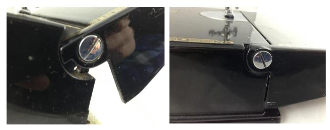
A difference in the rear folding bed hinge shape is illustrated above. This machine also has a small hole located in the hinge area that doesn't seem to appear on standard production machines, represented in the right hand photo by an early production AD series machine.
