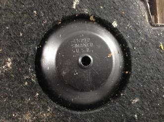
Also notice the indented area where the retention screw seats. The cover on this machine has a dome shaped indent while others I have observed have a more angular transition to a flat bottom as shown on the right.
