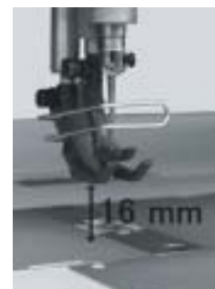
The clearance under the presser foot (16mm)
