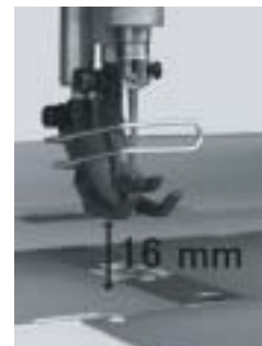
The clearance under the presser foot (16mm)
