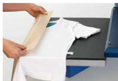
3 Make sure to apply the elements from the recommended side and use the correct pressing aid. To protect the heating surfaces from any glue residue, it is best to cover them with Teflon® film.
