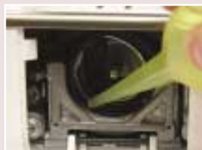
Oiling the oscillating hook system
