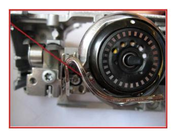
3. Bring the thread forward to the metal curve and to the highest point of the curve
