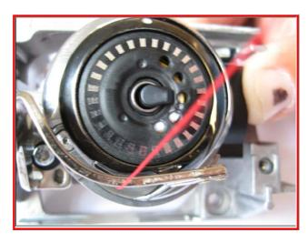
5. As you near the end of the retaining wall, you will feel a click and the thread has slid into the extra tensioner (slot) needed for embroidery.
