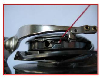
This is the slot the thread is going into. There is a mirror that came with the 830 to see this. Once you know the motion, the mirror is not necessary
