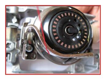
4. Let the thread slide down the metal piece (retaining wall)
