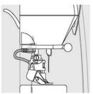
aurora 430/440: The BSR symbol will appear on left side of display screen, and presser foot icon will indicate Foot #42 (BSR). Press the BSR/Balance button; Mode 1 or Mode 2 – whichever was used last – will be selected, with stitch length set at 2.0 mm (if machine has not been turned off, settings will automatically return to the ones last used with the selected Mode). Stitch length may be adjusted from 1-4 mm.
