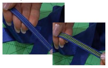
Not all sergers will be able to do all stitch types. It depends on the machine and the number of threads. These stitches can also be used in various combinations. On the Baby Lock Triumph, this results in 87 different stitch combinations.
