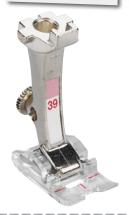
Sometimes called an appliqué foot, this foot was designed for satin stitching of all types. The sole allows satin stitches to pass under the foot evenly without building up and inhibiting the feed. Helpful red lines on the sole act as a visual guide for perfectly placed stitching!
