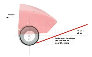
Cars will be towed up the ramp after each race, so a tow hook (eye bolt) should be provided for the tow strap. The hook must meet the clearance requirements outlined above.
