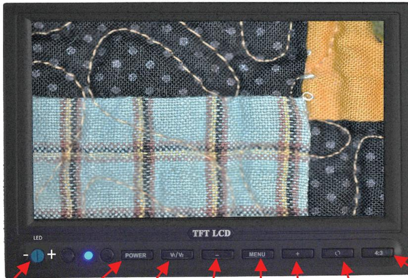
**LED Adjustment Power Un-used Down Menu Up Image Rotation 4:3/16:9**
