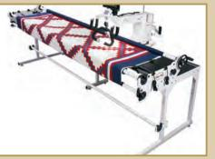
From its height-adjustable legs to the simple assembly and snap-in rail system, the Baby Lock Pearl Frame is the perfect accompaniment to the Crown Jewel. The work area is also adjustable—quilters can work with a 5 foot work space or increase it to 10 feet for larger projects. Add the
