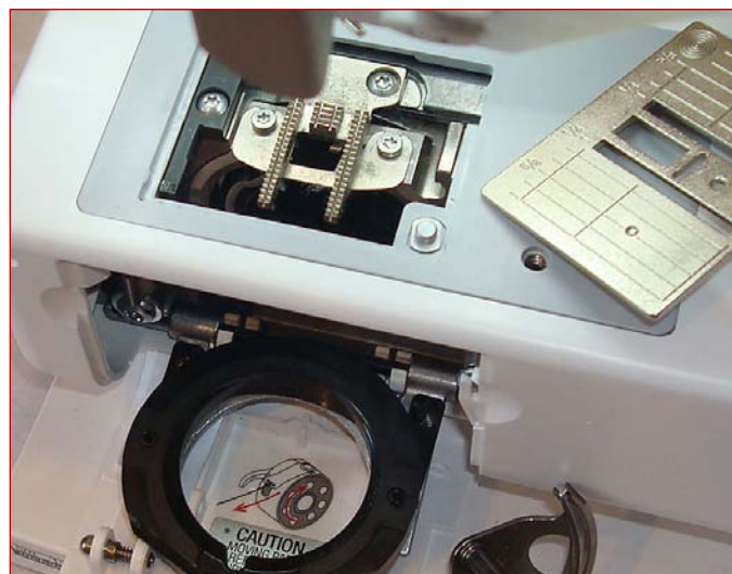
Remove stitch plate, bobbin case, and hook.
