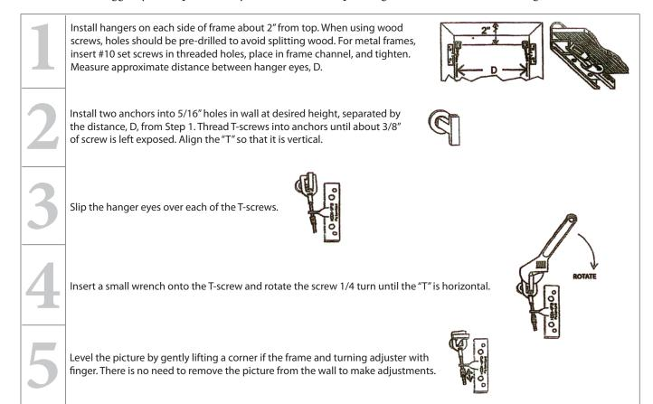
Tools you will need: Drill with 5/16 drill bits (masonry bits if you are drilling into brick or block), driver attachment for your drill to make the screwing go a lot faster (or you can use a screwdriver if you don't have one), a card-board box to use as a table top while you are mounting the hangers on the frames or plaques (this helps to not scratch the front of the frame or plaque), a hammer to pound in the mollies and a crescent wrench to turn the T-bolt.
